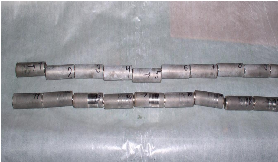
FIG. 2. The tube pieces with deposits after cutting.
