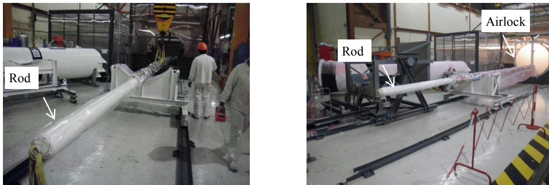
FIG. 7. Work airlock used to sample the rod (views from outside).
