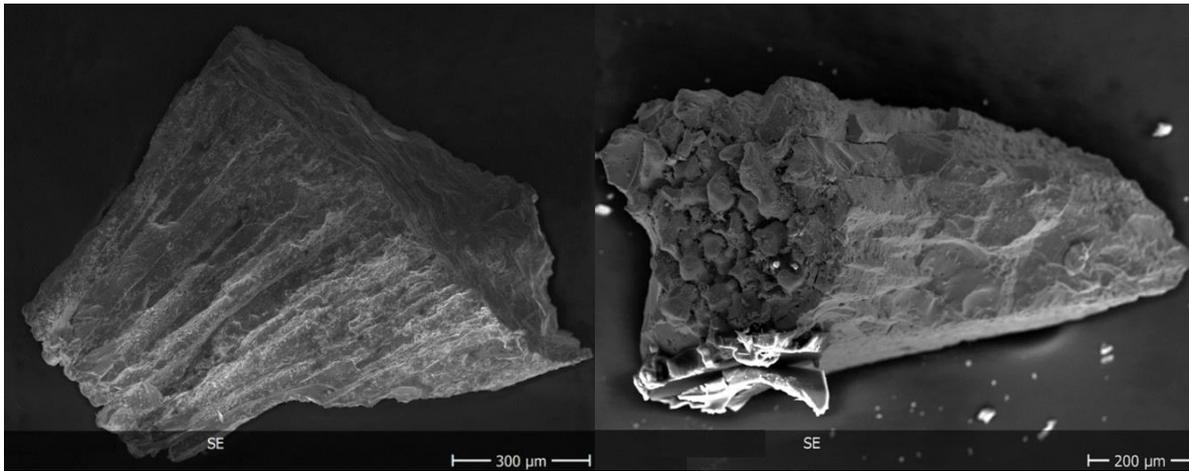
FIG. 2: SEM picture showing the microstructure of the fuel from the central hole to approximately the mid-radius. Left: radial view. Right: view from the central hole position
