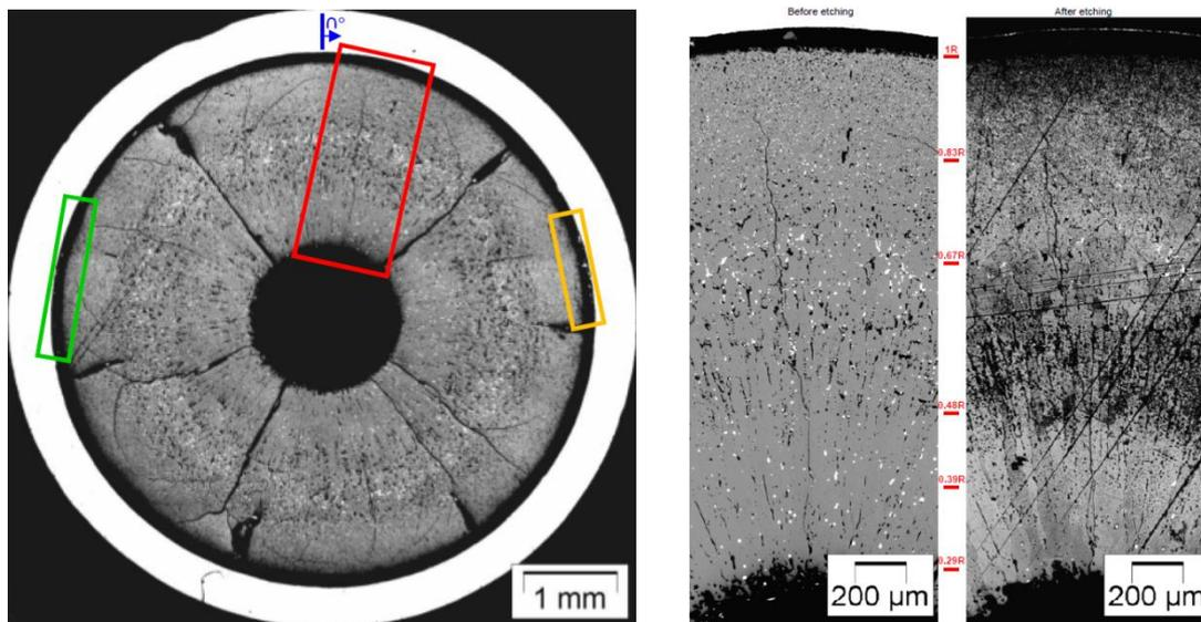
FIG. 1: Macrograph showing the complete fuel section and detailed view, obtained at the LECA star facility in CEA Cadarache.
