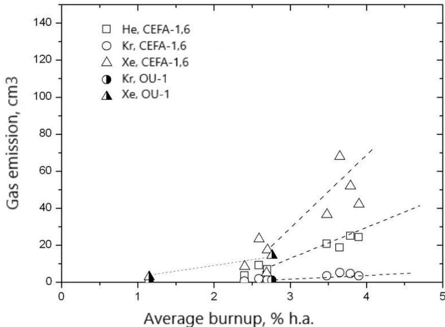
Figure 6 – Gas release from the nitride of BOR-60 EFA-1 (OU-1), CEFA-1 and CEFA-6 of BN-600
