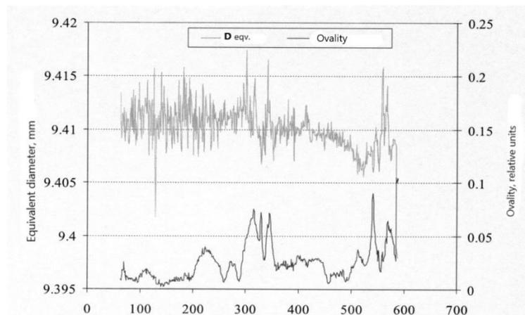
Figure 4 - Diameter and ovality changes of the cladding along the length of the fuel element of BOR-60 EFA-1 with a maximum burn-up of 1.3at%
