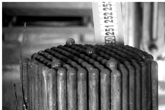
Figure 5 - Top end of CEFA-1 after irradiation in BN-600. (Values in Figure 5 note the numbers of fuel elements with nitride fuel.)
