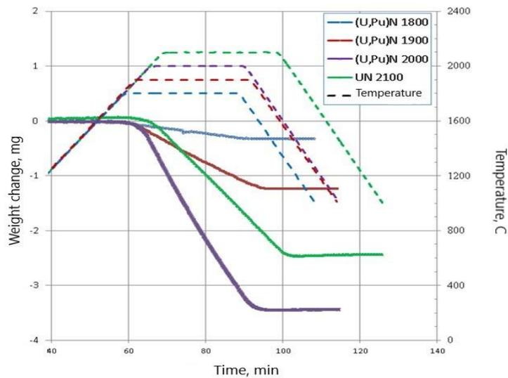
Figure 3 - Results of thermogravimetric researches of uranium nitride at the temperature of 2100°C and mixed uranium-plutonium nitride ( $U_{0,5}Pu_{0,5}N$ ) at temperatures 1800°C, 1900°C and 2000°C.
