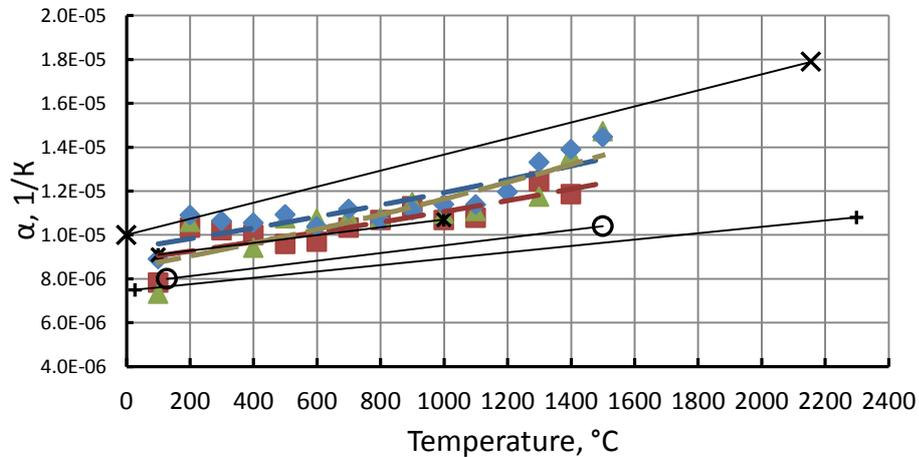
Figure 2 - Dependence of the linear thermal expansion coefficient of the samples:  $\blacklozenge$  ( $U_{0,95}Pu_{0,05}N$ ),  $\blacksquare$  ( $U_{0,90}Pu_{0,10}N$ ),  $\blacktriangle$  ( $U_{0,85}Pu_{0,15}N$ ) from the temperature (the limit of the permissible relative tolerance of measurements of linear increments is 3%) in comparison with the literature data [2].
