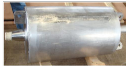
Fig. 2 : Manufactured Submersible ALIP with outer stainless steel enclosure
