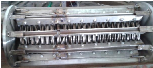
Fig. 1: Submersible ALIP with MI Cable winding and CRGO laminations
