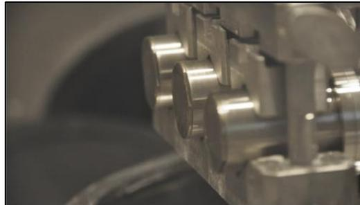
FIG. 5 : Ultrasonic transducers being developed for under-sodium NDT (TUCSS)
