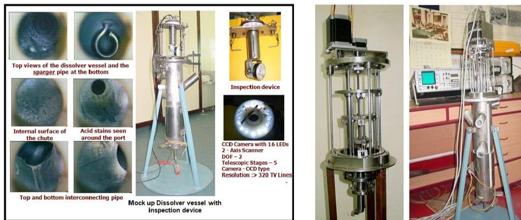
Fig.5 Remote inspection of CORAL dissolver vessel
