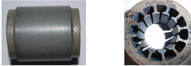
Fig.4 Rotor and stator of centrifugal extractor with PEEK coating
