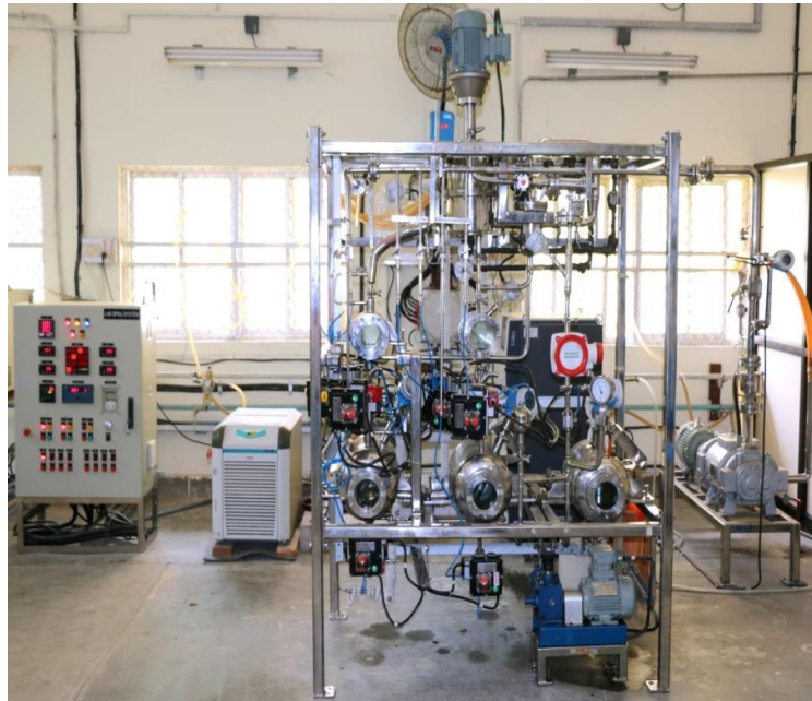
Fig.7 Solvent purification system
