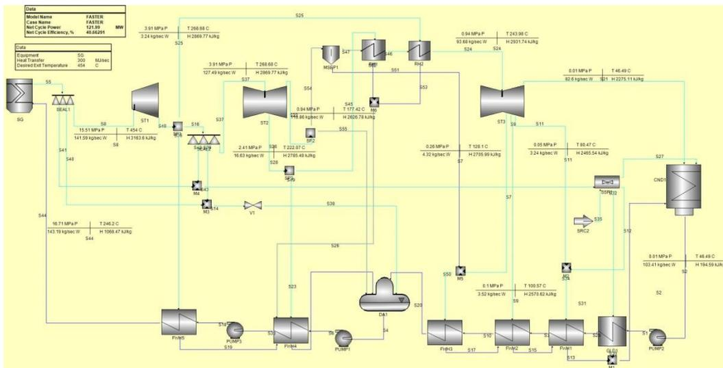
Figure 4 – FASTER Thermodynamic Cycle and Balance of Plant
