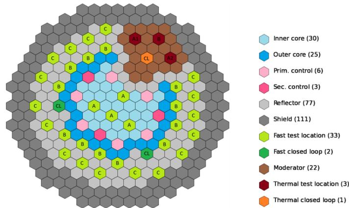
**Figure 1 – FASTER Reactor Core Layout**
