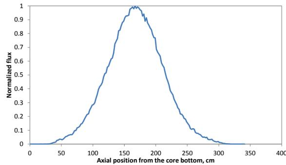
**Figure 6 – Normalized axial thermal flux distribution in the test locations**
