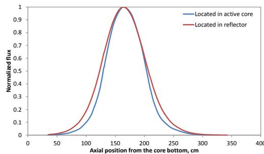
**Figure 5 – Normalized axial fast flux distribution in test locations**
