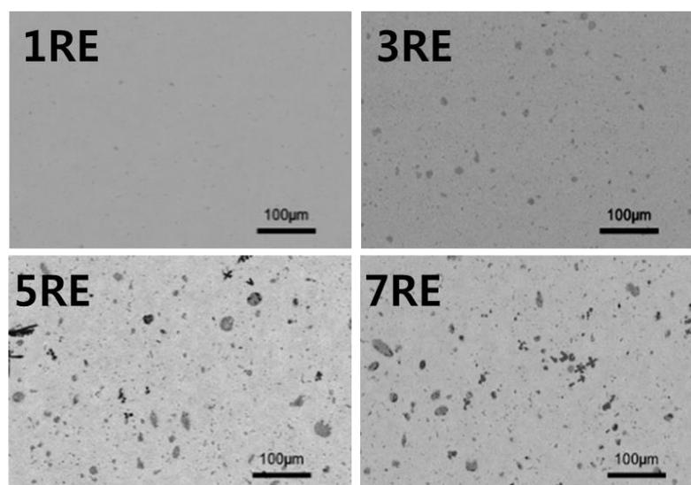
FIG. 3. Scanning electron micrographs of U-10wt.%Zr-(1,3,5,7)wt.%RE alloys fabricated by the injection casting
