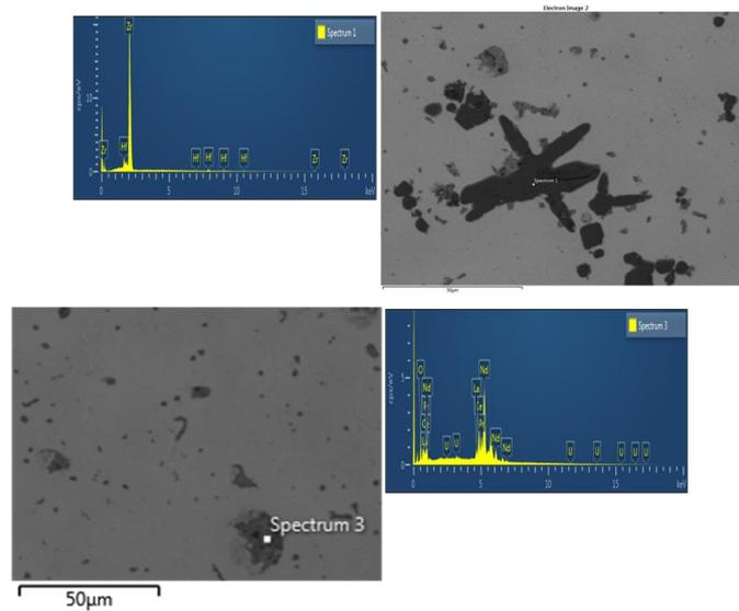
FIG. 4. EDS results on inclusions formed in U-10wt.%Zr-5wt.%RE alloys fabricated by the injection casting
