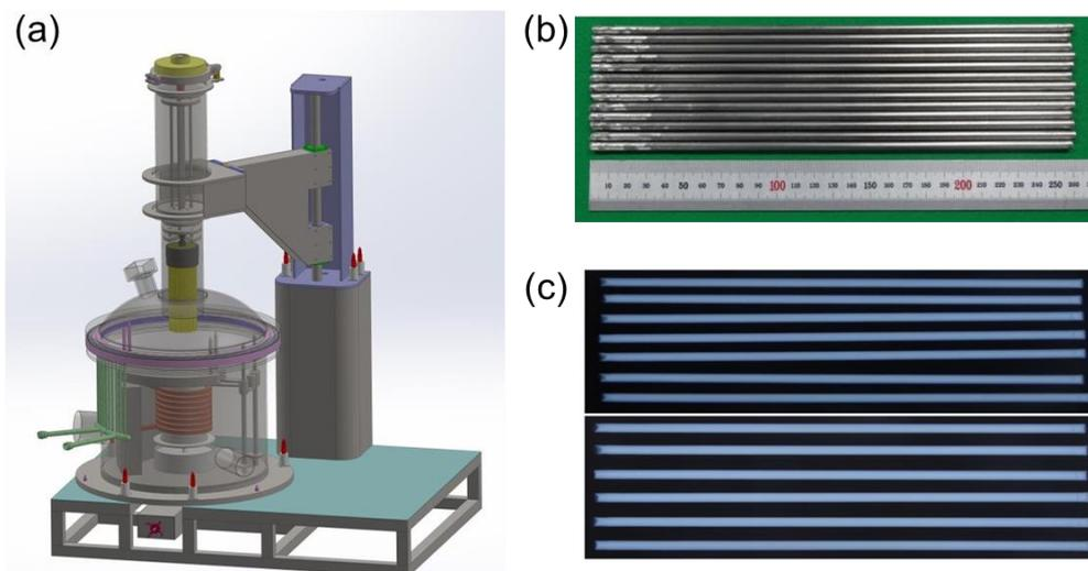
FIG. 1. (a) Schematics of injection casting furnace, (b) U-10wt.%Zr fuel slugs fabricated by the injection casting and (c)  $\gamma$  ray radiographs for the fabricated fuel slug.
