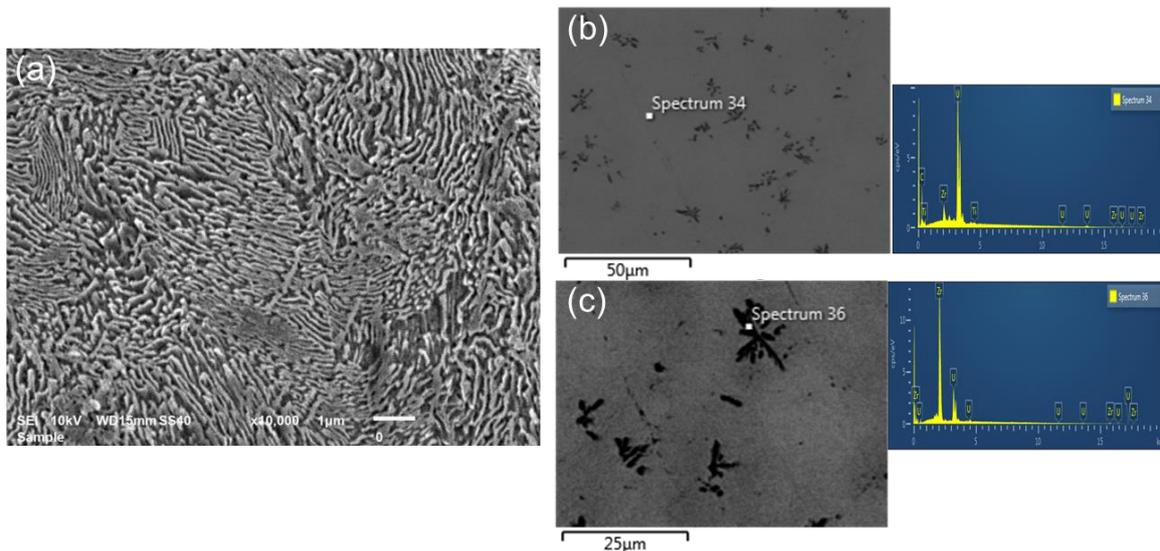
FIG. 2. (a) Scanning electron micrograph showing a lamellar structure of U-10wt.%Zr fabricated by the injection casting and EDS results on (b) the matrix and (c) inclusions.
