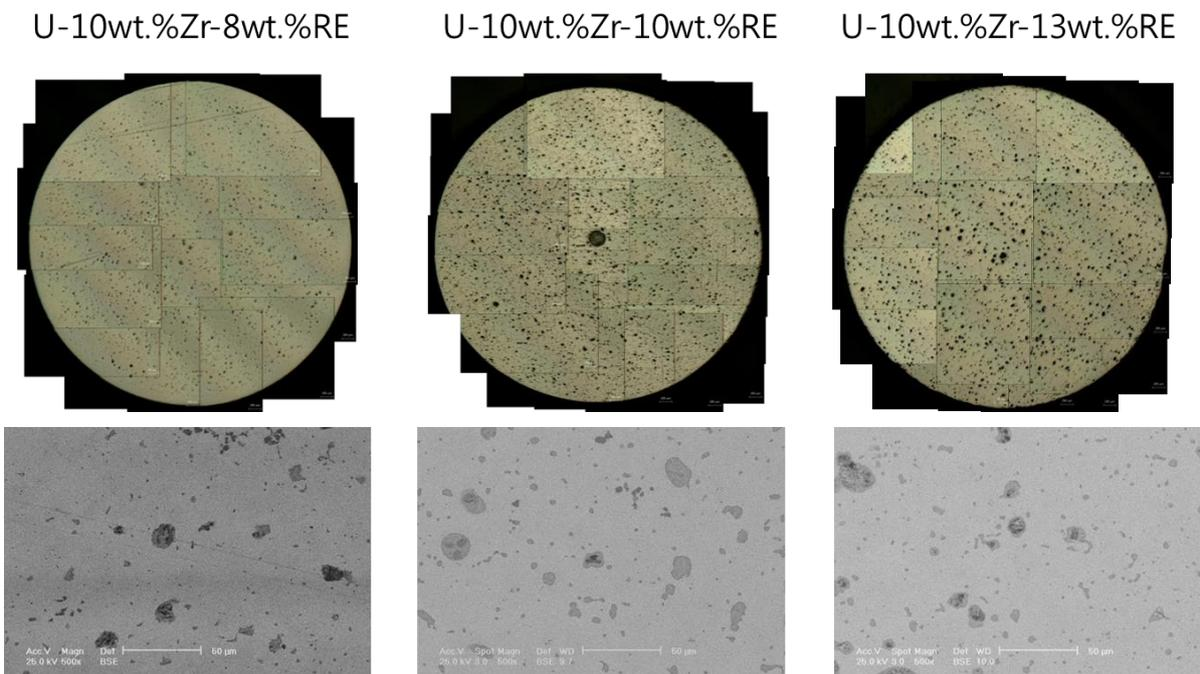
FIG. 5. Optical and scanning electron micrographs of U-10wt.%Zr-(8,10,13)wt.%RE alloys fabricated by the injection casting
