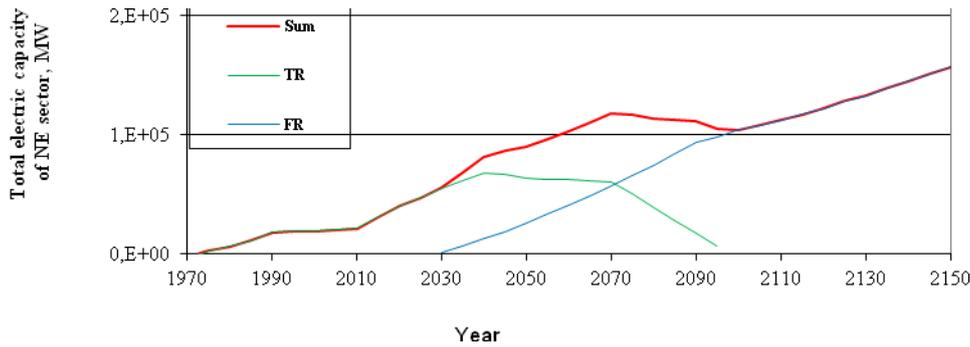
Fig.8. Model scenario of nuclear power development in RF.
