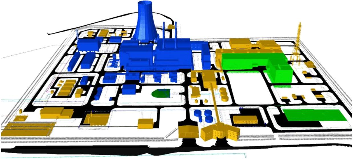
*Fig. 1. PDEC general scheme of phased commissioning: yellow – fabrication/refabrication facility – first stage, blue – BREST-OD-300 reactor unit – second stage, green – SF recycling and RAW handling facility.*
