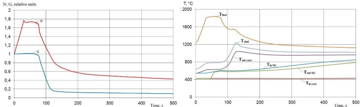
Fig. 6. Major reactor characteristics change under UTOP.
