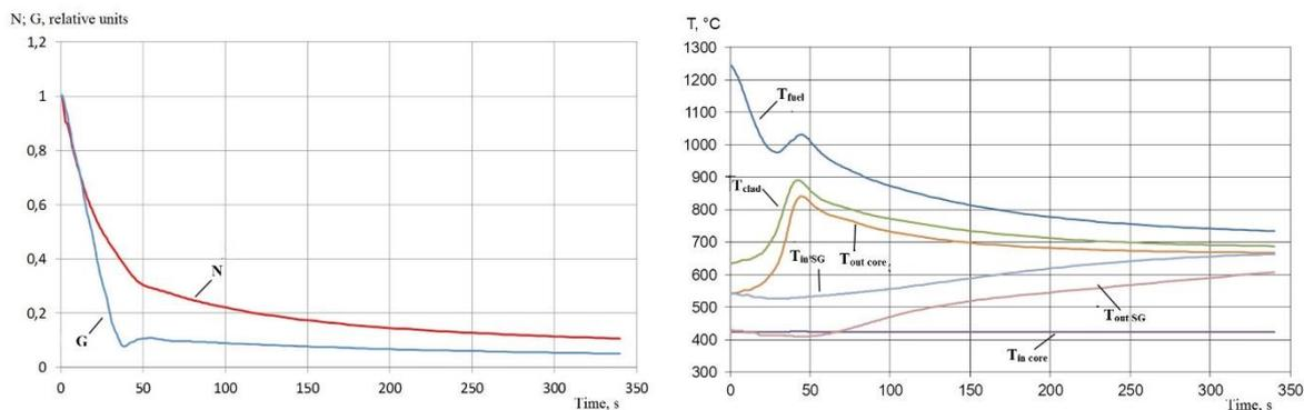
Fig. 5. Major reactor characteristics change under ULOF.
