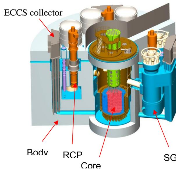
*Fig. 2. Integral design scheme of BREST-OD-300 reactor unit.*
