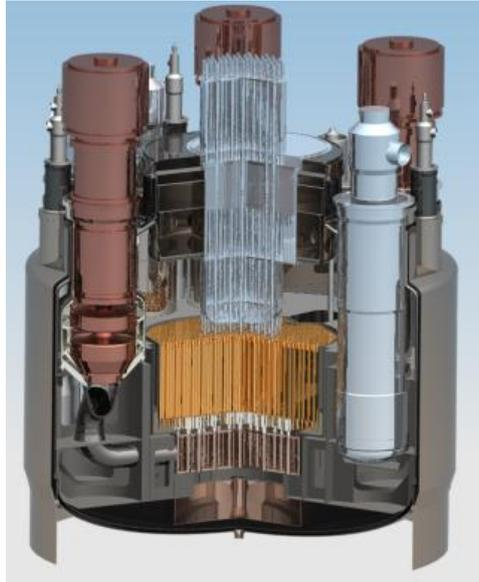
*Fig. 10. BN-1200 reactor layout.*
