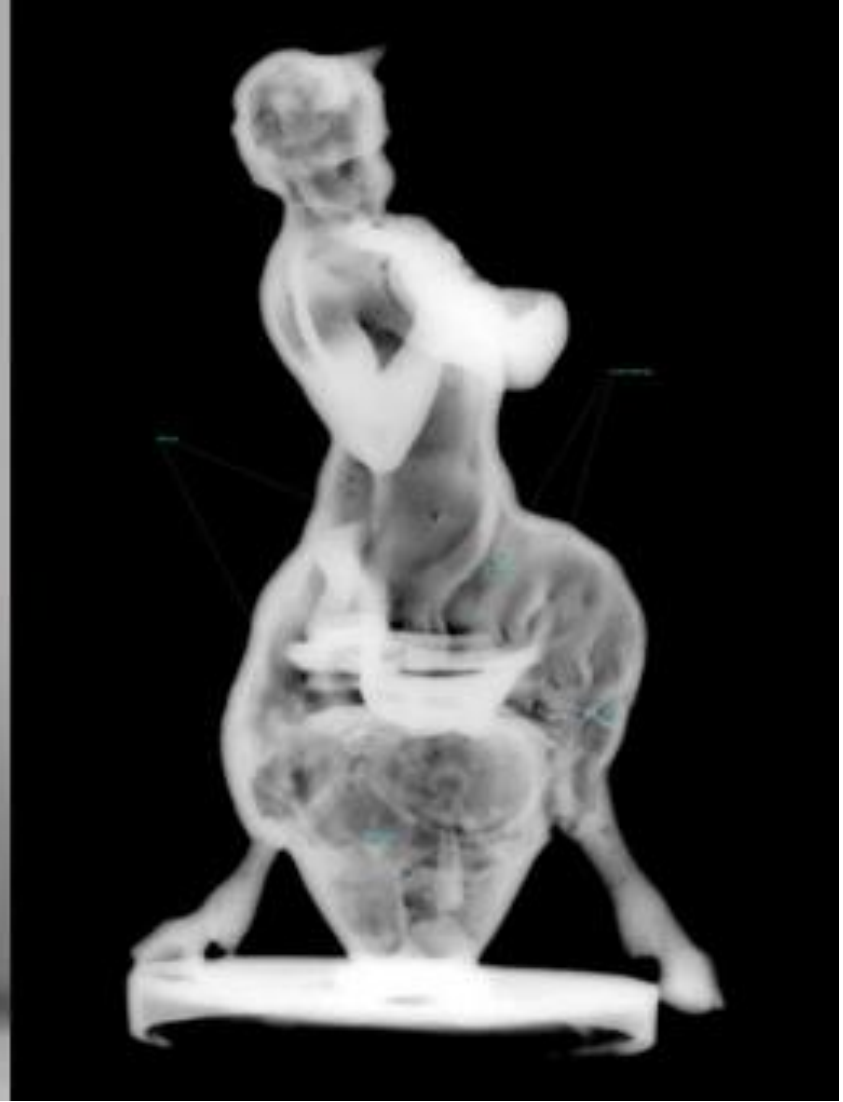
Example of radiography with imaging plate: Satyr with Urn (Walters Art Museum, Baltimore - MD). Italian sculpture, 16 th century. Photography & radiography with imaging plate GE-CR50P. The X-ray image reveals wax drippings and circular metal plugs
