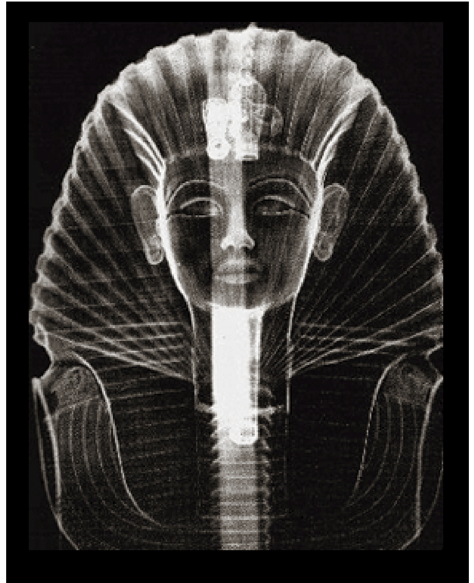
Gamma radiography (iridium 192 - Kodak Définix film) of the Gold mask of Tutankhamon , at the occasion of the exhibition «Tutankhamon et son temps» - Petit Palais Paris (1967) - © SGS - Qualitest
