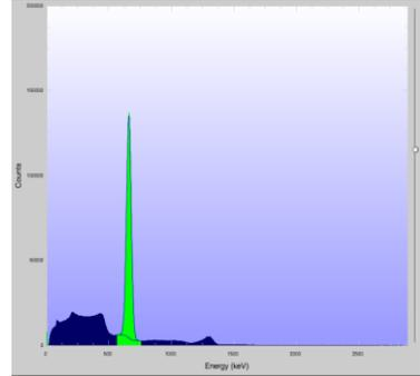
The counts generated at **energy peak-660KeV for Cs-137** (marked as green in the fig) is taken for analysis purpose.
