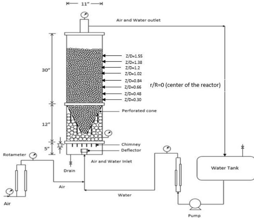
Schematic diagram of lab scale upflow packed/expanded bed reactor
