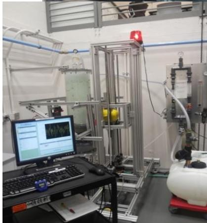
For Pinpointing Flow Pattern (Regime), Radial/Diameter Profile of Phases' Holdups
