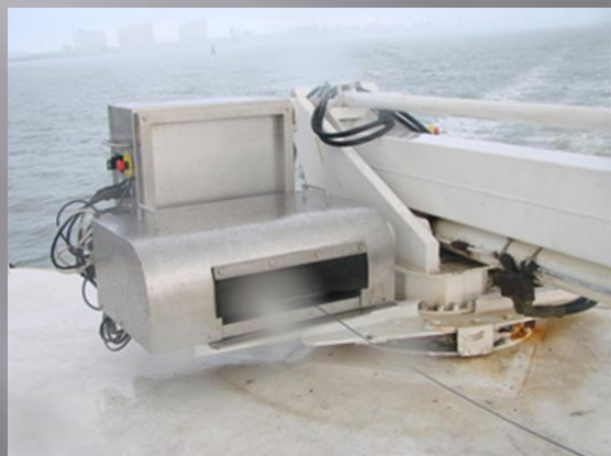
Winch SAR IV : 220 VAC - 2 kW - 2 speeds (max 2 m/s) - max load 150 kg
